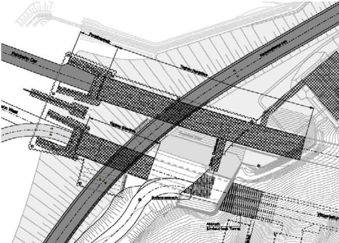
Figure 4. Construction phase A.1 with traffic trough the old tunnel (top) and C.1 after opening of the north tube (bottom).
